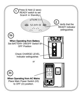
Figure 12. ScanX Power Shut Down
