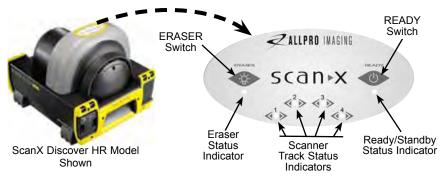
Figure 5. Membrane Keypad and Indicator Locations
